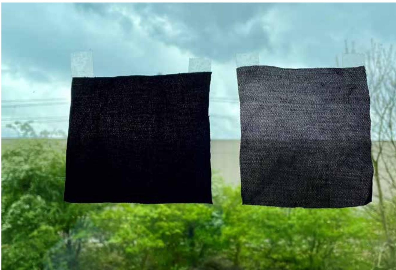
*Light transmission through fabric treated and untreated.*
